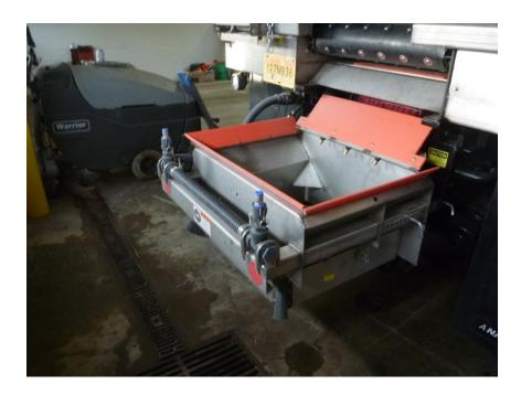
430 gallon tank installed inside the truck body
