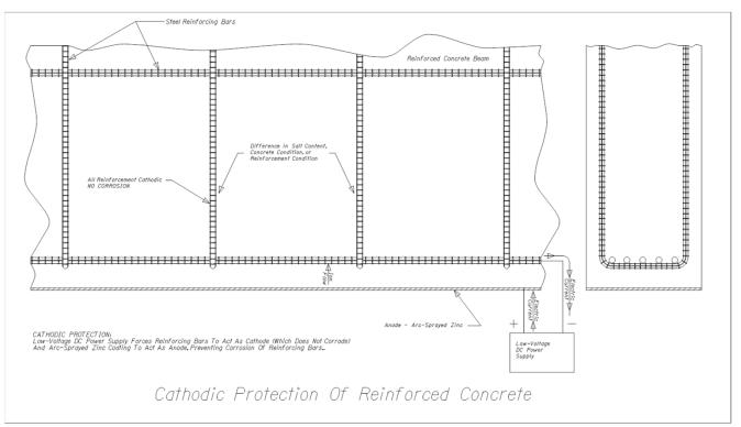
ODOT's Bridge Preservation Program was founded in the 1980s to save historic coastal bridges using impressed current cathodic protection. Low-voltage direct current passes from the zinc coating on the reinforced concrete surface to the reinforcement, driving corrosion to occur at the zinc coating rather than the steel.
