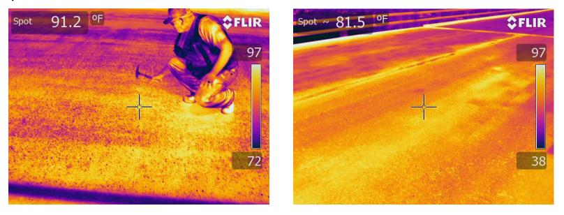
Delaminated areas heat up faster during rising temperature and cool down faster during dropping temperature. These images were taken in the morning.
