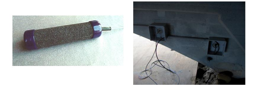
Includes installation of reference cells for future corrosion monitoring.
